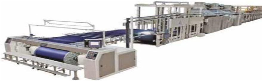
Indigo Slasher Dyeing & Sizing machine
